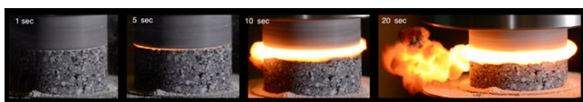
Fig. 1: Freeze-frames of a HVR experiment performed on a basaltic-andesite; one sample applies axial load and the other rotates (here 2 MPa, 1.4 m/s).
